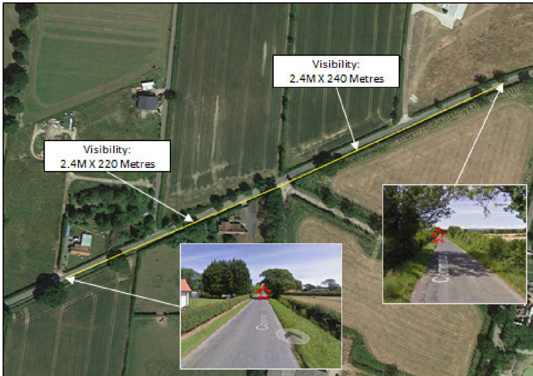
Figure 1: Visibility of Access on Common Lane
